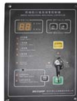
Bridge Navigational Watch Alarm System
